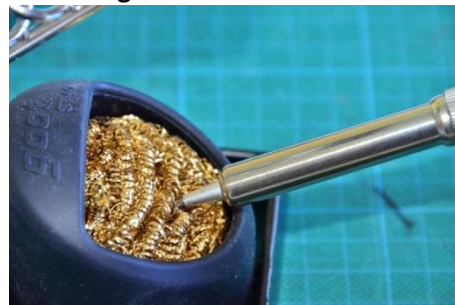
Poke the tip in and out several times
