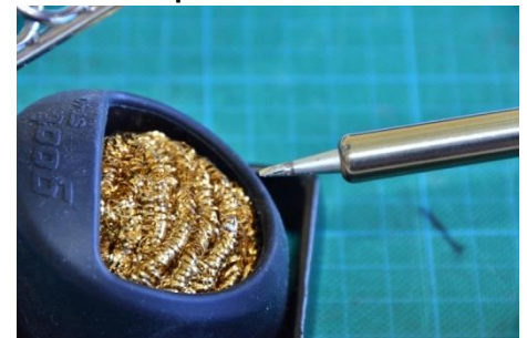
Check the tip is shiny and clean
