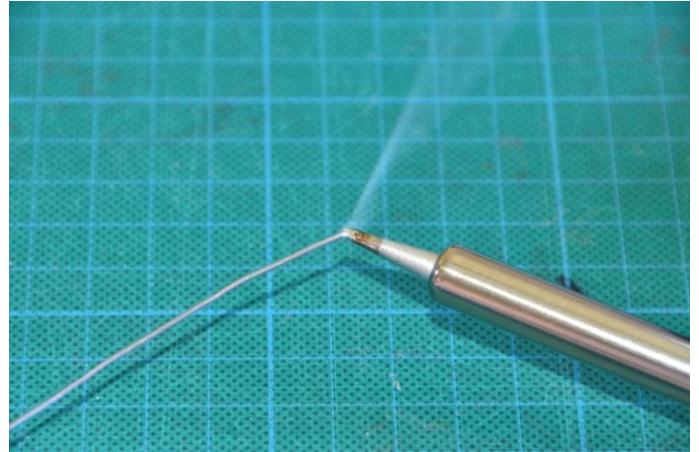
Melt some solder onto the tip. The flux will smoke.
