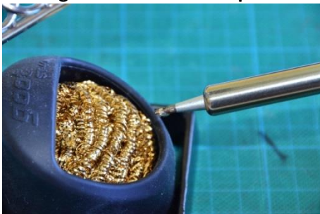
Bring the tip close to the tip cleaner
