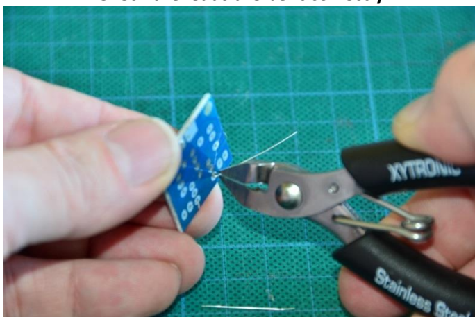
Cut the other lead the same way
