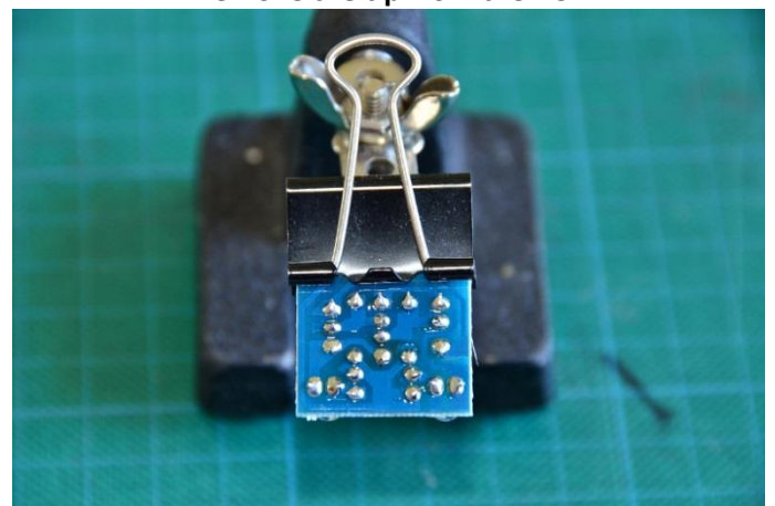
Check all pads are soldered and shiny
