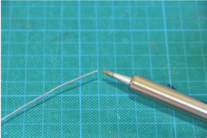
Bring the solder to the tip of the hot soldering iron
