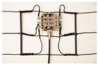
The 1:1 parallel transmission-line current baluns and the autotransformer were all made by winding 1.25mm enamelled copper wire on Amidon FT140-43 toroidal, ferrite cores, which can each handle 100W or more. An insulating sheet is also placed between the cores to discourage any arcing. The autotransformer has 13 turns with taps at 8 (80m), 10 (40m/Feed) and 13 (20m).
